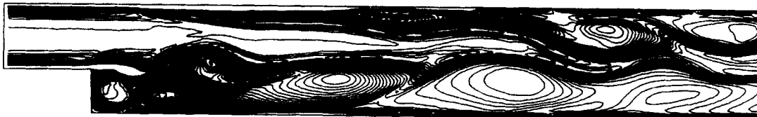
Figure 14. Vorticity contours for unsteady flow in backward-facing step
